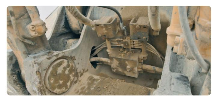
The electrical HCC hose connection control is a monitoring and signalling unit to reliably check lubricant feed lines for breaks. This unit shows the driver or operator of the machine immediately if there is a fault by sending a collective fault signal.
